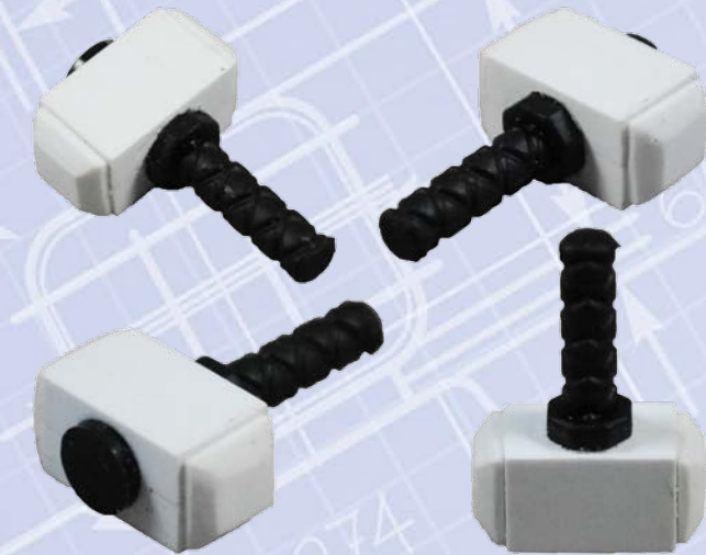
Prototype: Custom prototype element for molding created with sheet styrene.
